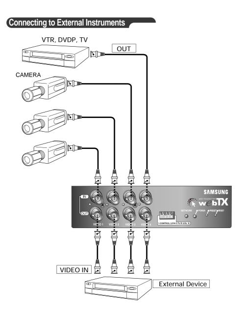
SNS-110 produces the video image signal of the corresponding channel, if connected with external instruments to Video Out 1~4 (loop through BNC). The terminal resistance of  $75\Omega$  will be automatically seized by the connection with external instruments.
